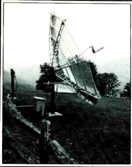
Figure 2: Paracclipse™ 3.8 m (12-foot) mesh antenna used in this user report.
