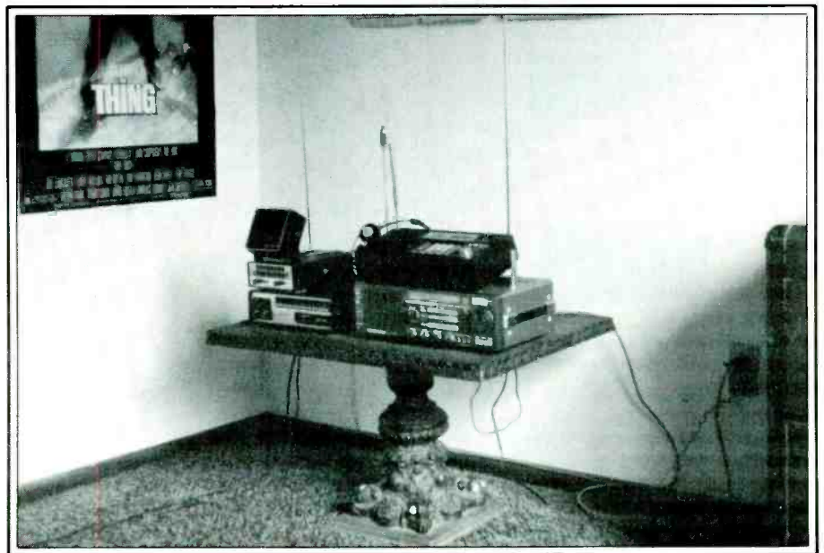
The author's equipment, used for deep sea monitoring, includes an R-2000 Trio-Kenwood communications receiver, a Radio Shack Comp-100 scanner and a DX-400 shortwave radio.
